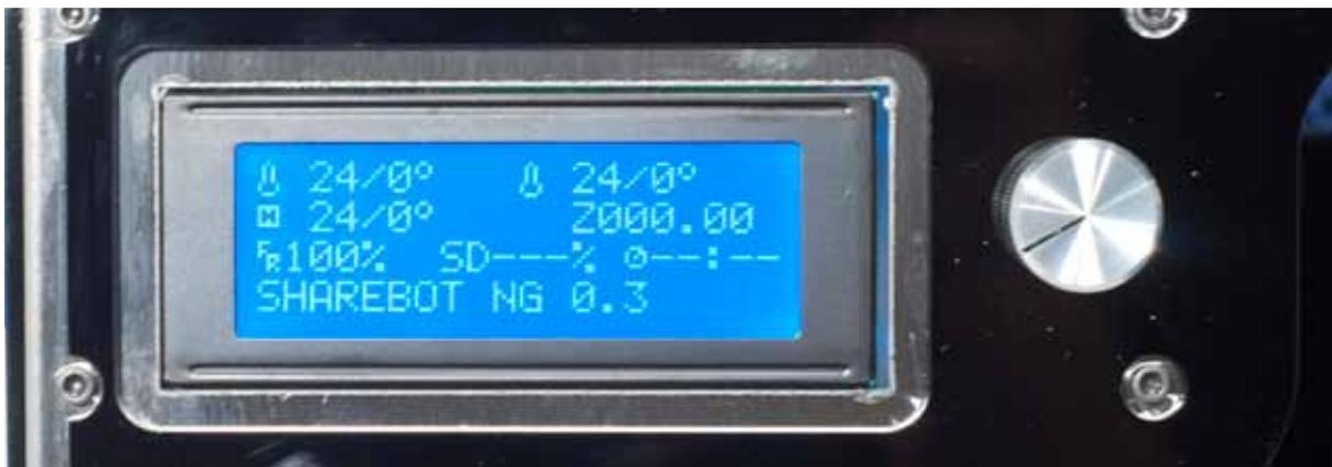
The first line contains the actual extruder temperature followed by one set; If the extruders are two, the first is on the left while the latter is right. What is used as the primary extruder is the one on the right. The temperature is in degrees Celsius.
